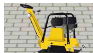
Vibratory plate (with newbuilds)
